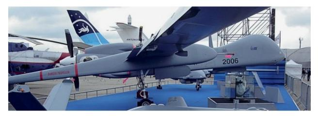
The Israeli drone Heron TP can stay in the air for up to thirty-six hours, fly at a maximum speed of 230 miles per hour, and carry more than a ton of cameras and bombs. (IAI)
